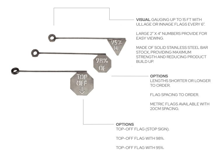
The GUARD LEVEL® Visual Gauge Tree (VGT) is a radial gauge tree which, when used with sight glasses, provides enhanced gauging ability for full depth gauging. Its unique design allows for absolute tank level readings and visual gauging up to 15 feet, clearly marked with ullage or innage flags every six inches or optional metric versions (available with 20cm spacing).
