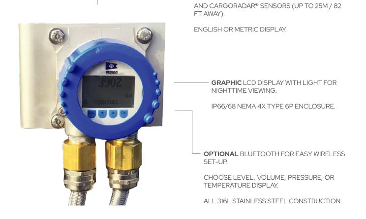
The GUARD LEVEL® Remote Display Unit (RDU) is a series of rugged remote display instruments made in two distinct models – RDU-81 and RDU-82 – with different connection options. The RDU-81 is specifically designed for the CARGORADAR® units and uses a 4-wire connection. The RDU-82 is similar to the RDU-81 except it is designed as a universal display for any 4-20mA/HART type 2-wire sensor making it ideal for remote display for the Hydrostatic Pressure Transducer (HPT) series of pressure sensors.
