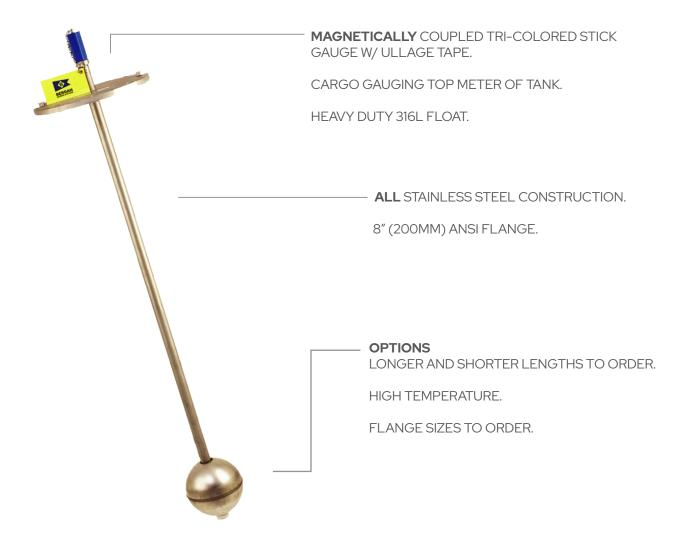
The GUARD LEVEL® Magnetically-Coupled Dip Stick (MDS) is a magnetically coupled gauge-stick giving a visual reference on tank barges during loading for designated "Safe" or "Hazardous" areas complying with all Code of Federal Regulations. Its rugged, stainless-steel design and simplicity of operation assures safe loading and prevention of tank overfills – with over 14,000 units currently in service.
