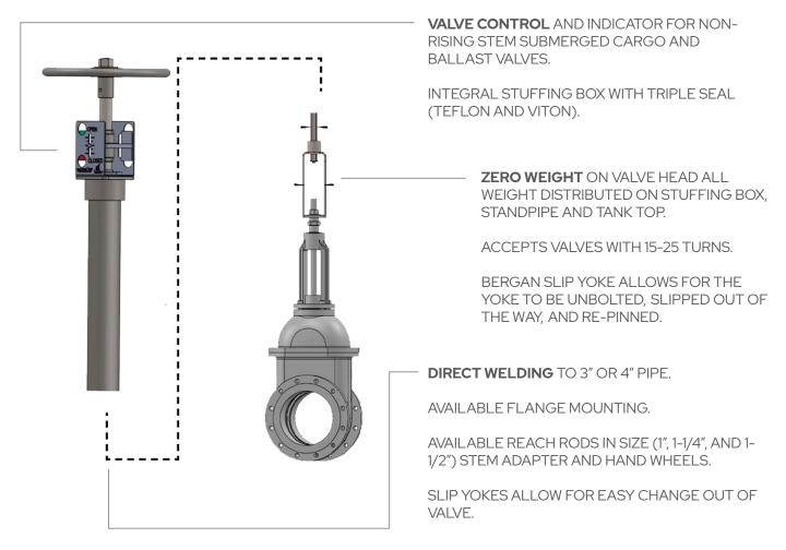
The GUARD VALVE® series of products are designed for manual control of non-rising submerged cargo and ballast valves and give a clear indication of the valve position even from afar.
