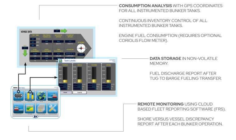
The GUARD LEVEL® Fuel Management System (FMS) is an inventory management system for tug boats and other smaller crafts that produces an audit trail to easily optimize fuel usage and reduce and eliminate fuel pilferage. This intuitive tank gauging system has extended hardware and software capabilities.
