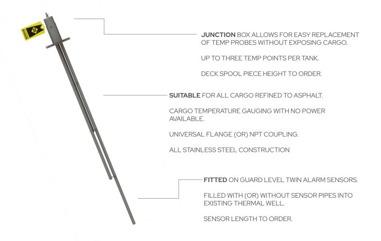
The GUARD TEMP<sup>™</sup> Barge Cargo Temperature Unit (BCTU) is a rugged low-cost stainless-steel tank temperature sensor designed for tank barges providing fast, accurate measurements and – the biggest advantage – no more mess. To add to the convenience, the unit requires no permanent cabling and is easily installed in any tank opening of two inches or larger.
