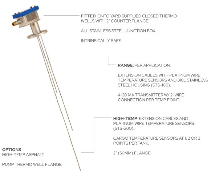
The GUARD TEMP<sup>™</sup>Single Temperature Sensor (STS) series of tank temperature sensors are designed for tank ships and tank barges and can be fitted at one, two or three points per tank – with pump thermo well flange or high temp asphalt options.
