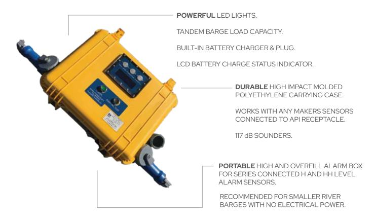
The GUARD LEVEL® Portable Alarm Unit (PAU) is a rugged portable solution for on-board alarm annunciation on inland and coastal river barges. The system monitors and raises alarms through series-connected alarm sensors and gives a unique warning for both High Level (HL) and Overfill Level (HHL). This battery-powered unit plugs into existing tank barge API receptacles. It complies with all CFR regulations for tank overfill control.
