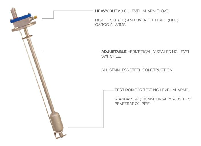
The GUARD LEVEL® 07324 MKII is a highly reliable and simple level alarm sensor for tank barges and tank ships. The MKII has an enviable record of providing the ultimate defense against tank overfill conditions. The alarm sensor can be applied as either a single or dual alarm point (1A or 2A) utilizes the proven principle of a float with magnetic actuation of a highly reliable bi-stable dry switch contact. With a built-in test rod, full functional testing can occur before loading tank.
