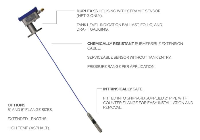
The GUARD LEVEL® Hydrostatic Pressure Transducer (HPT) series are rugged stainless steel, Intrinsically Safe sensors that easily and accurately measure pressure readings in any tank environment. From high pressure full fuel oil tanks to tank vapor line lower pressure situations, the sensors work to assure ease and high accuracy, with safety first on the list. And, for all sensors, pressure ranges can be set according to your exact specifications.
