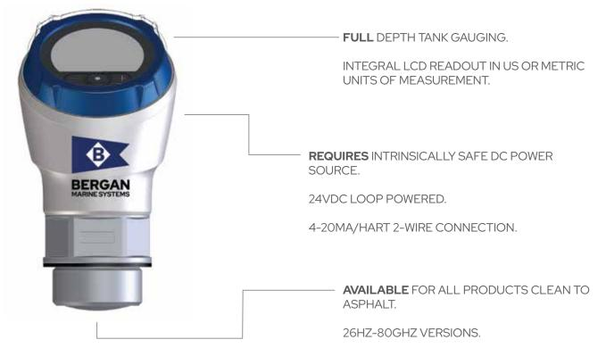
The CARGORADAR<sup>®</sup> series is a mainstay for your tank gauging needs. Through our OEM Vega Americas' partnership, we've produced a high tech, high accuracy (+/-2mm) non-contact ullage measuring instrument. From 6GHz to the latest 80Ghz tightly focused Frequency Modulated Continuous Wave (FMCW) radar transceiver, the CARGORADAR<sup>®</sup> is perfect for any tank gauging applications with multiple mounting options.
