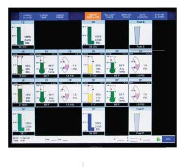
**SUMMARY** SCREENS FOR SERVICE TANK, BALLAST TANK, CARGO PRESSURE, PUMP AND MANIFOLD, CARGO ULLAGE, AND CARGO TEMPERATURE.
