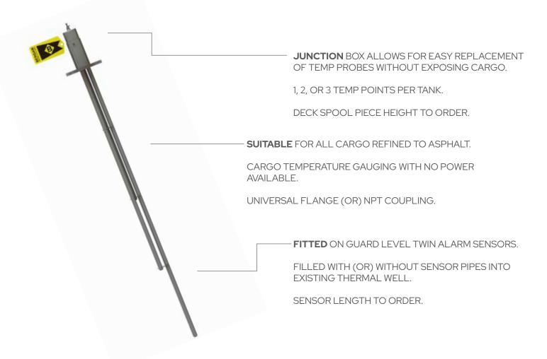
The GUARD TEMP™ Barge Cargo Temperature Unit (BCTU) is a rugged low-cost stainless-steel tank temperature sensor designed for tank barges providing fast, accurate measurements and – the biggest advantage – no more mess. To add to the convenience, the unit requires no permanent cabling and is easily installed in any tank opening of two inches or larger.
