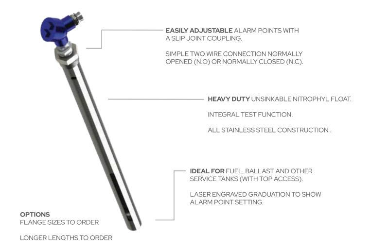
The GUARD LEVEL® Adjustable Compact Alarm Sensor (ACLAS) is an ingenious way to assure overfill protection on bunker tanks and other small service tanks accommodating a variety of setups. Its rugged stainless-steel single alarm point level sensor fits into any tank opening of 1.5 inches (G1.5) or greater, while its dry reed switch opening allows for either an Normally Closed (N.C.) or Normally Opened (N.O.), allowing for simple sensor interface to any alarm system.
